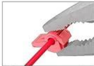
03. Squeeze the connector together until it locks
